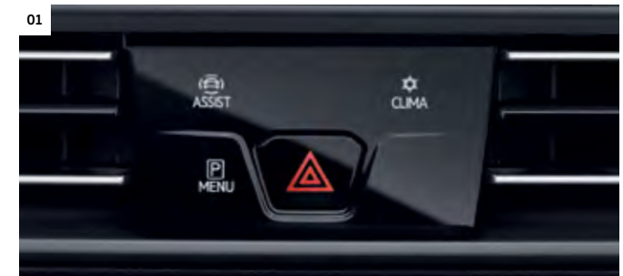
01 Direct access button module. The module is arranged centrally around the hazard warning lights button and uses shortcuts for easy access to major functions such as driver assistance systems, air conditioning functions and parking assistance systems. | C | L |
